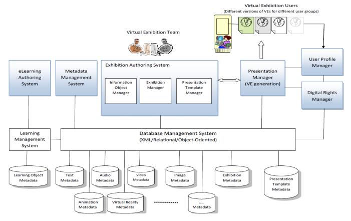
Figure 2. Generic system architecture for VE development
