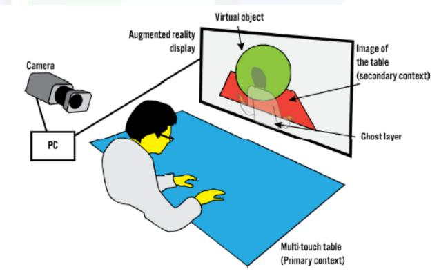
Fig. 1. Setup of Multi-touch augmented reality system
