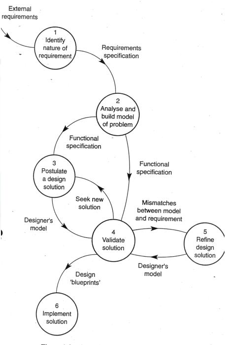
Figure 1.2 A model of the design process.
