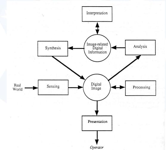
Figure B.1 - Computer imaging model
