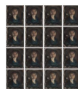
Figure A2. Images of daguerreotypes scanned with different light modes. From left to right: LRFB, LR, LFB, LF, LTx, LTx 5cm, LTx 10cm, RTx, RTx 5cm, RTx 10cm, LLa, LRFB 15deg, LR 15deg, LFB 15deg, LF 15deg, L 15deg.
