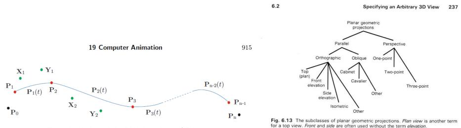
Figure 19.1: An Interpolating Bézier Curve for n + 1 Points.
