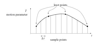
Figure 13.2: Motion control by interpolation
