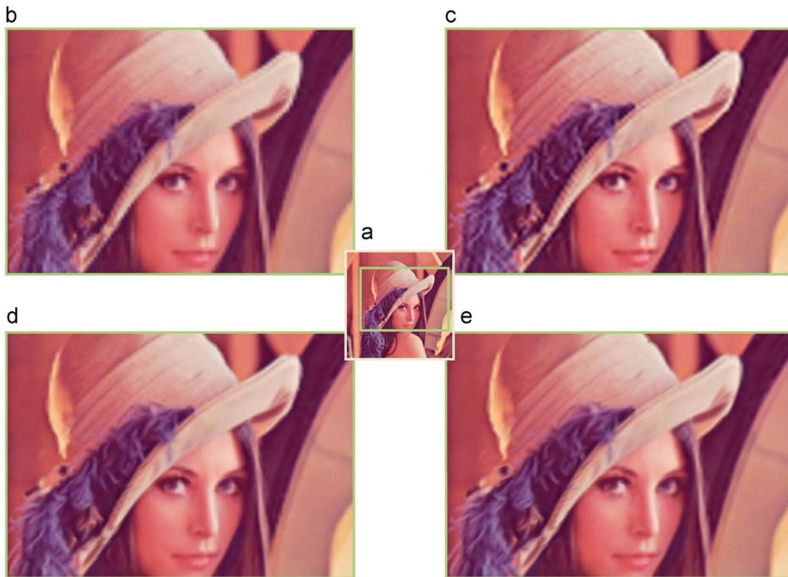
Fig. 12. Reconstruction results at 400 percent magnification: (a) original image; (b) bilinear filter; (c) Lanczos filter; (d) CPU-based DDT and (e) GPU ExpROI2 Max Gain modification.
