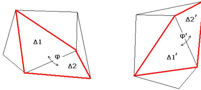
Figure 4.3: Strictly similar patches - Two strictly similar patches are marked with red - they must fulfill the following requirements:  $\Delta_1$  and  $\Delta'_1$  must be strictly similar,  $\Delta_2$  and  $\Delta'_2$  must be strictly similar,  $\varphi = \varphi'$  angle between the planes containing  $\Delta_1, \Delta_2$  and  $\Delta'_1, \Delta'_2$  respectively
