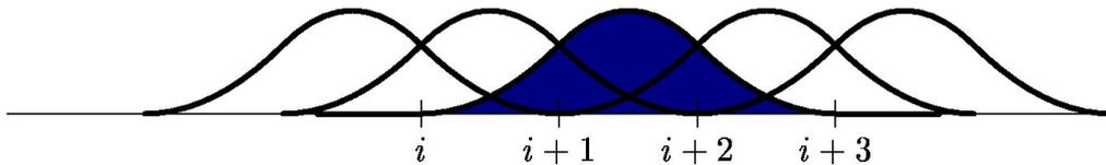
Figure 3.3: Uniform quadratic B-spline basis function
