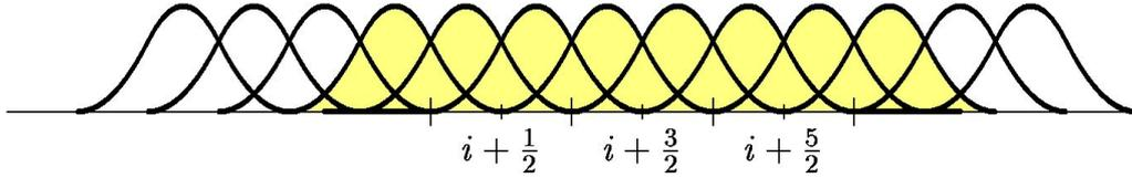
Figure 3.4: Uniform quadratic B-spline basis function defined over refined knot sequence
