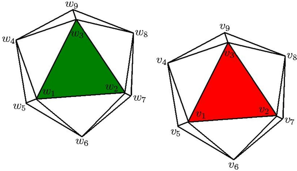
Figure 4.2: Topological conditions for the Loop scheme
