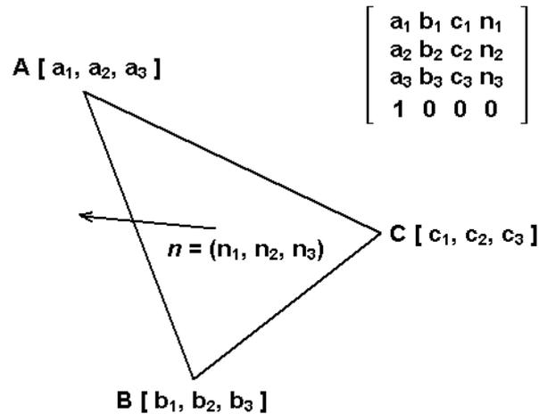
Figure 4.4: Matrix describing the position and orientation of a triangle
