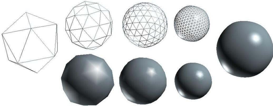
Figure 3.1: An example of Loop's subdivision scheme applied on a very rough geosphere (4 iteration steps are shown - left: the initial mesh, middle: 3 successive refinement steps, right: the 4th level of the subdivision )
