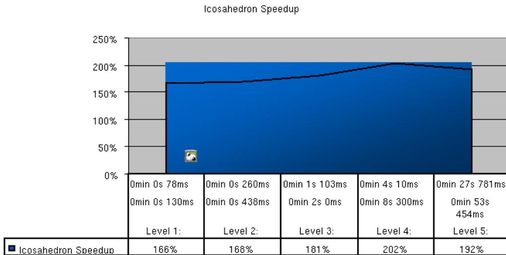
Figure 4.6: Time needed for processing subsequent levels of subdivision steps. The best result is achieved by subdividing the 4th level: the speed is more than doubled
