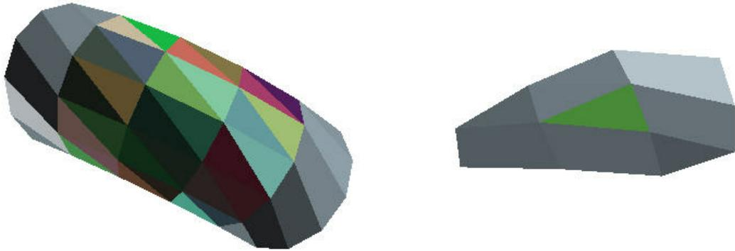
Figure 4.9: On the left: set of triangles of a torus needed to reproduce the mesh - result gained by using the vector  $(1,0,0,0,0)$  On the right: the same torus can be reproduced from one single triangle - using the vector  $(0,0,1,0,0)$
