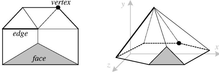
Figure 2.4: Cell complex and its corresponding mesh
