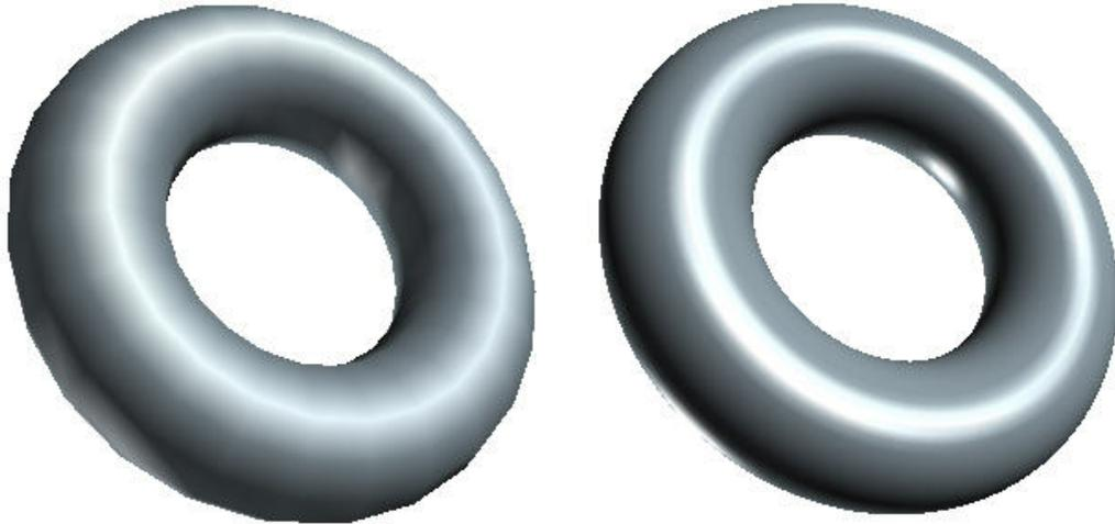
Figure 4.7: On the left: picture of a torus in the initial form (437 faces). On the right, the torus is subdivided 2 times (16393 faces)
