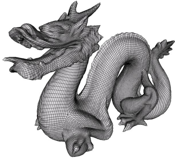
Figure 12: A remesh of the genus 1 dragon. Remeshing the original scanned dragon with genus 46 would be nearly impossible, given the difficulty of achieving a high-quality parameterization for high-genus models.
