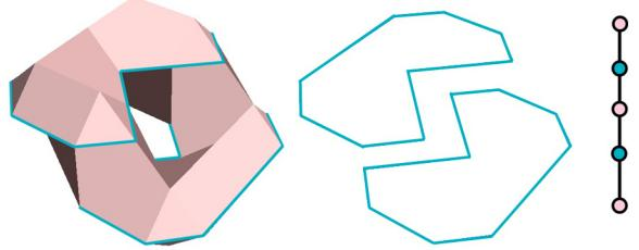
Figure 7: Example of intra-ribbon handle. This torus tilted at an angle is formed by two “C” shaped contours. As shown on the right, the Reeb graph does not contain any cycle.
