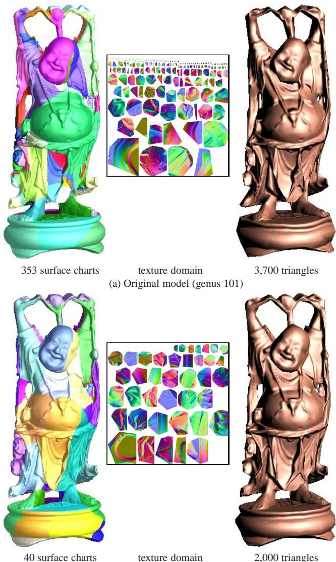
Figure 15: Comparison of normal-mapping progressive meshes before and after topology simplification. Both models refer to 512x512 texture images. The topological complexity of the original model requires many more parametric charts, shown in pseudocolor. The resulting fragmentation of the parametric domain restricts simplification.
