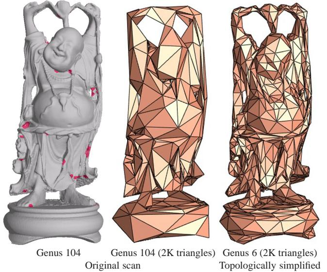
Figure 1: This scanned Buddha mesh has genus 104 instead of the expected 6. Regions with extraneous handles are highlighted in red. The two images on the right compare mesh simplification results before and after topology simplification. The high-genus mesh requires many triangles to needlessly represent topological artifacts, resulting in loss of overall geometric quality.
