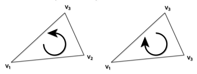
$\square$  Compute normal:  $n = (v_2 - v_1) \times (v_3 - v_1)$
