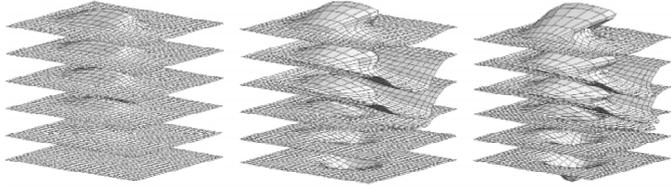
Figure 5. Coons body 2 with B-spline boundary surfaces. The de Boor points of boundary surfaces can deform the shape and interior of the original cube.
