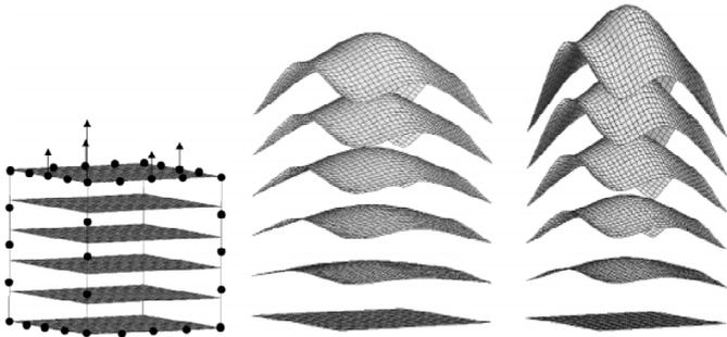
Figure 3. Coons body 1 with B-spline boundary curves. B-spline de Boor points along the edges deform the cube.
