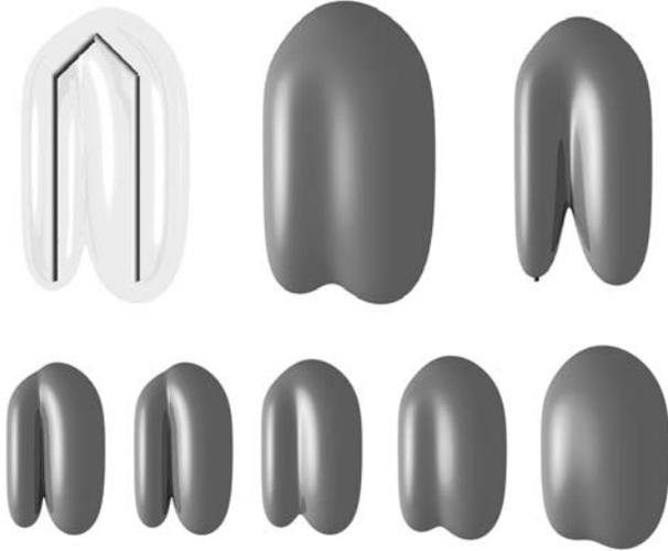
Figure 1: Blending union operation. top: standard and bottom: Blending union operation.
