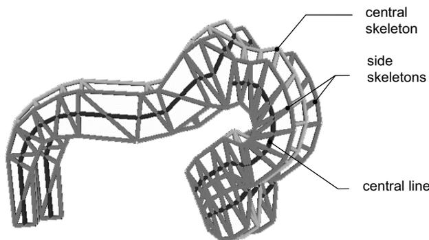
Figure 4: Adding the thickness by scaling and shifting the central skeleton.
