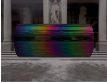
Figure 8. Chrome oxide thin film interference with increasing thickness from 100 nm to 400 nm.
