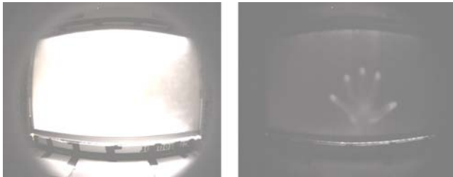
Figure 5: Captured image without infrared bandpass filter on the left, and with infrared bandpass filter on the right
