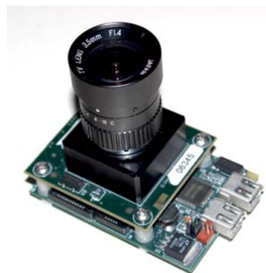
Figure 2: Firewire camera from Pixelink with wide angle lens mounted.
