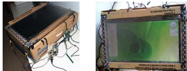
Figure 1: Current version of our prototype consisting of a LCD screen below a plexiglass which is edge illuminated with 850 nm infrared LEDs.
