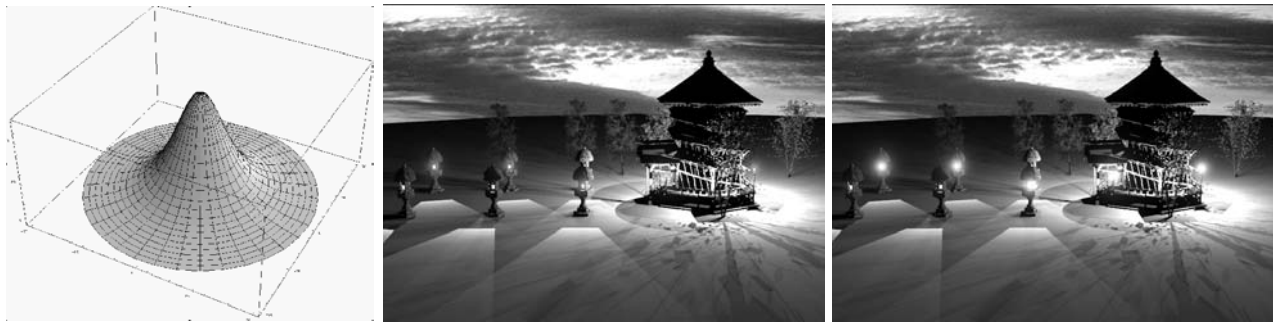
Figure 4: Camera bloom: left) the filter profile center) the scene without any effects right) the scene luminaries enhanced by a bloom effect.
