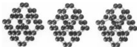
FIGURE 3 Oxygen and silicon interactions including two electron vacancies ( Si_{36}O ). The oxygen atom is located in the center.
