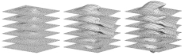
Figure 5. Coons body 2 with B-spline boundary surfaces. The de Boor points of boundary surfaces can deform the shape and interior of original cube.
