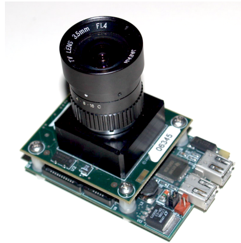
Figure 2: Firewire camera from Pixelling with wide angle lens mounted
