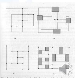
Fig. 1.6 (a) An orthogonal drawing, (b) a box-orthogonal drawing, (c) a rectangular drawing, and (d) a box-rectangular drawing.
