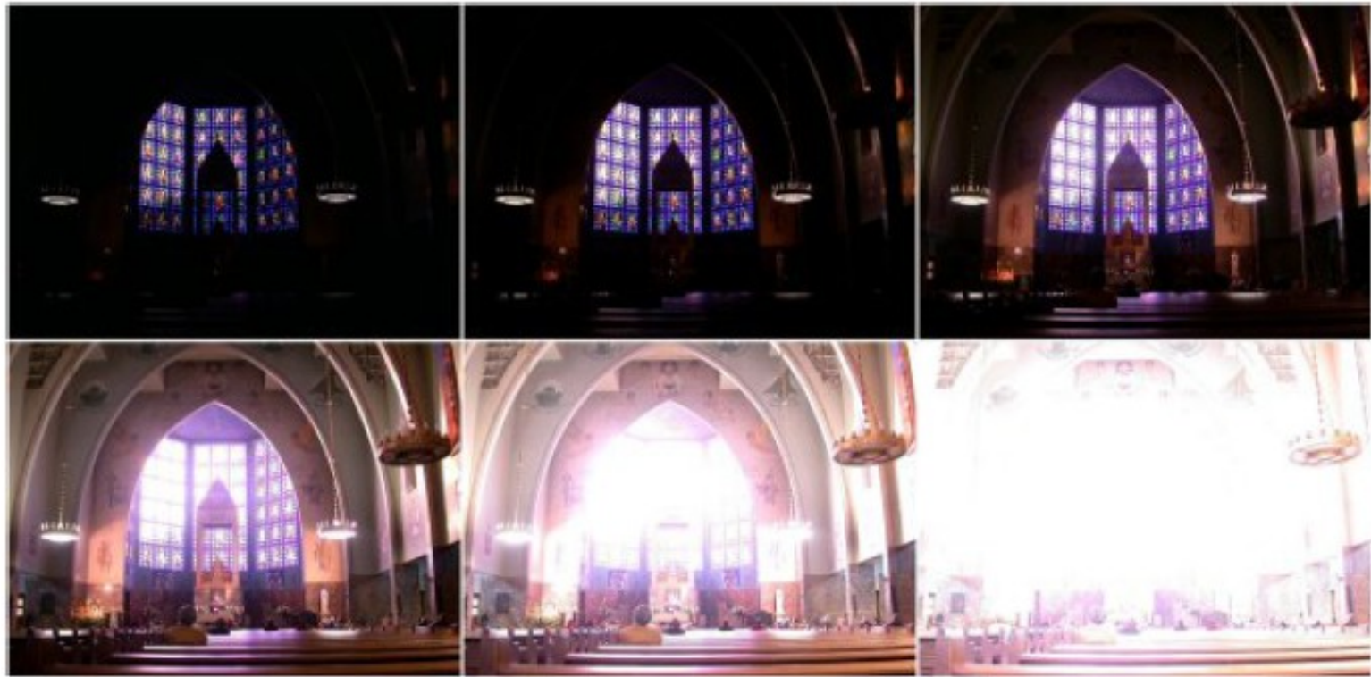
Figure 3: Sequence of exposure-bracketed image, separated by one f-stop. The shortest shown exposure time is 1/60 sec (top left), the longest 15 sec (bottom right). Aperture fixed at 2.6, ISO 100. Taken with Nikon CoolPix 995. Source: Axel Jacobs
