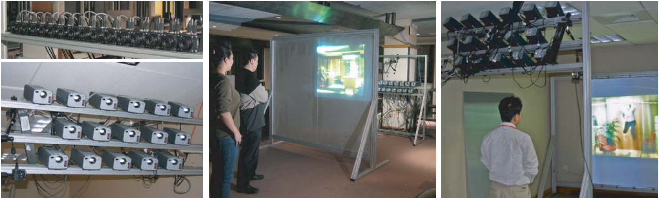
Figure 1: 3D TV system. Left (top to bottom): Array of 16 cameras and projectors. Middle: Rear-projection 3D display with double-lenticular screen. Right: Front-projection 3D display with single-lenticular screen.
