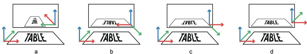
If the camera is placed behind the user, the projected image is an aligned extension of the 2D table space. Our experiments show that the users were able to operate the table top easily in this set-up even when looking at the augmented reality display instead of the table display. We argue that this improves the immersion and reduces the confusion when switching attention from one display to another.
