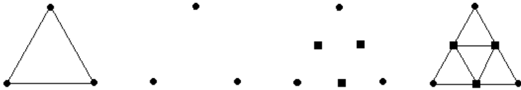
Figure 3 Topology refinement for one triangle and inserting new vertices.
