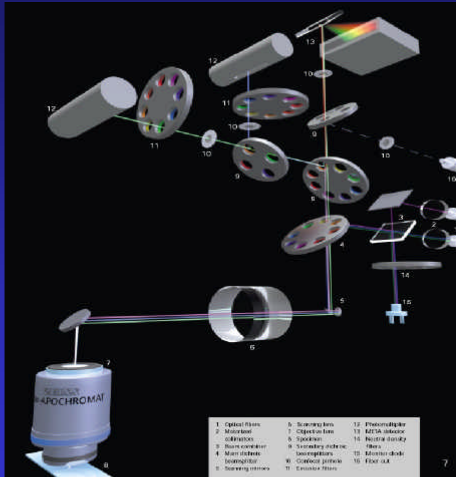
Optical scheme of LSM META 510
